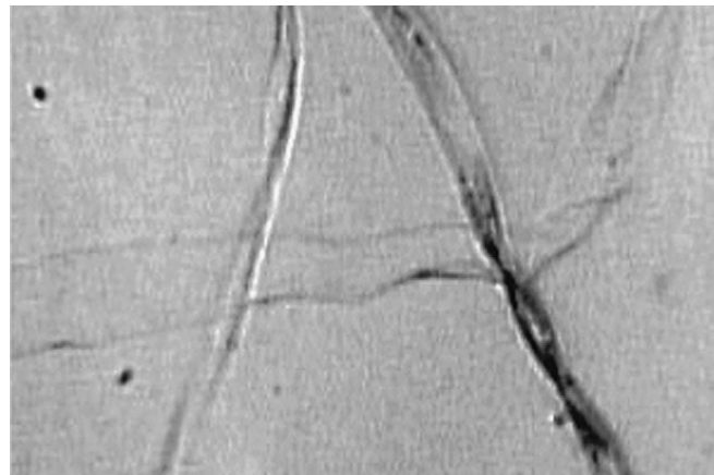
Fig. 7. Treated cotton sample in ionic liquid ([Bmim]+Br − ) seen by optical microscopy in transmitted light, T = 80\text{ }^{\circ}\text{C} .
